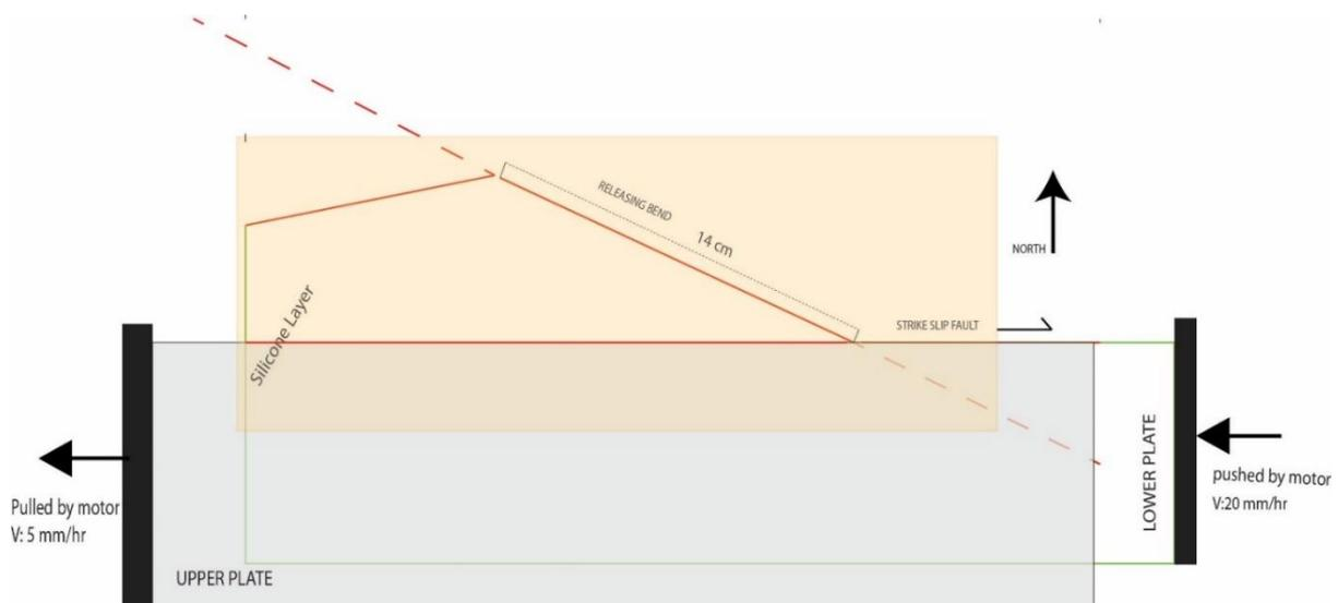
**Figure 1** showing the one of example of experiment setup of models
