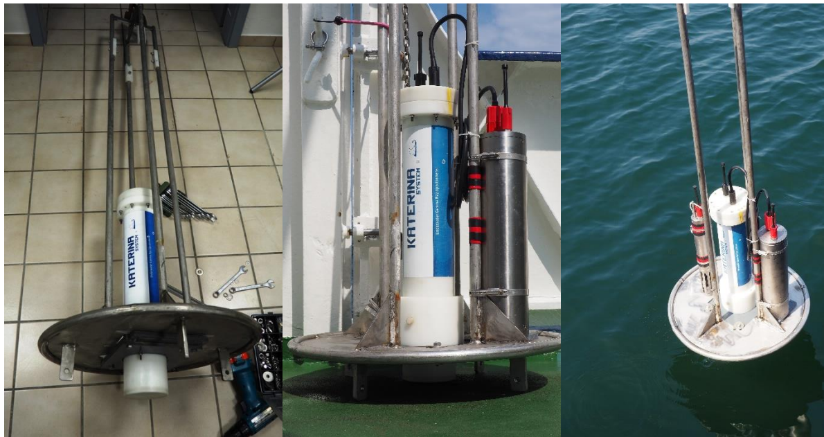
Figure 1. Adaptation of the gamma-ray spectrometer KATERINA onto application specified platform along with CTD meter and battery pack. Attention was paid to the proper exposure of the detection crystal to seawater and its protection from accidental bump on the seabed
